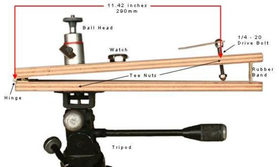
A 1/4 - 20 bolt is placed at exactly 11.42 inches, or 290mm, from the center of the hinge pin. When this bolt is turned at one rotation per minute, the camera will track the stars as they move across the sky. The tripod's adjustments are used to aim the axis of the hinge pin at the north celestial pole.
