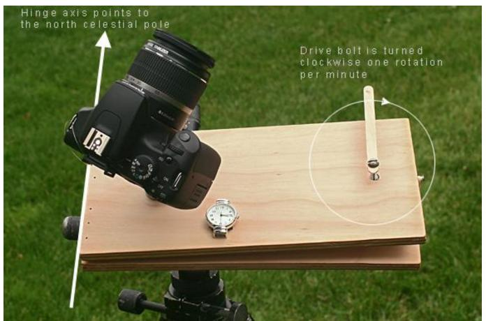
A simple barn-door tracker can be made for about \$15. The axis of the hinge on the left points to the north celestial pole near Polaris. The bolt on the right is turned one rotation per minute to drive the tracker to follow the stars.
